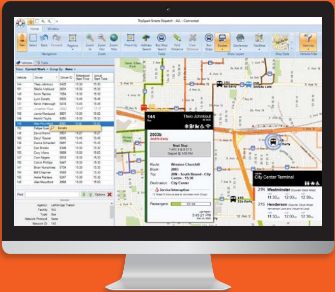
Streets Dispatch set-up viewed on a dual monitor system. Includes Streets Automatic Vehicle Locator (AVL), Computer Aided Dispatch (CAD) and Route Monitor windows.
